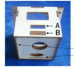
If you using the motor not listed this manual, make sure that when installed, The distance from the firewall to the drive washer to correctly match the cowl spacing, you can choose A or B.
