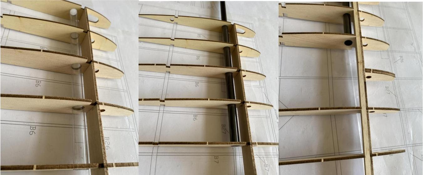
6) Glue reinforcing plates B27 on wing main girder splices, followed by installation of wing ribs.
