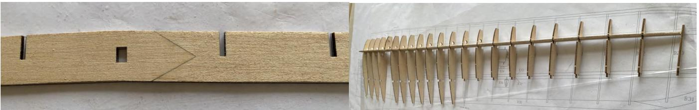
**5) Install PVC sleeves for positioning with carbon tubes, then glue balsa strips onto main beams.**
