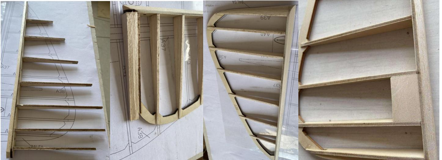
**2) Assemble the elevator ,using carbon tube positioning.**
