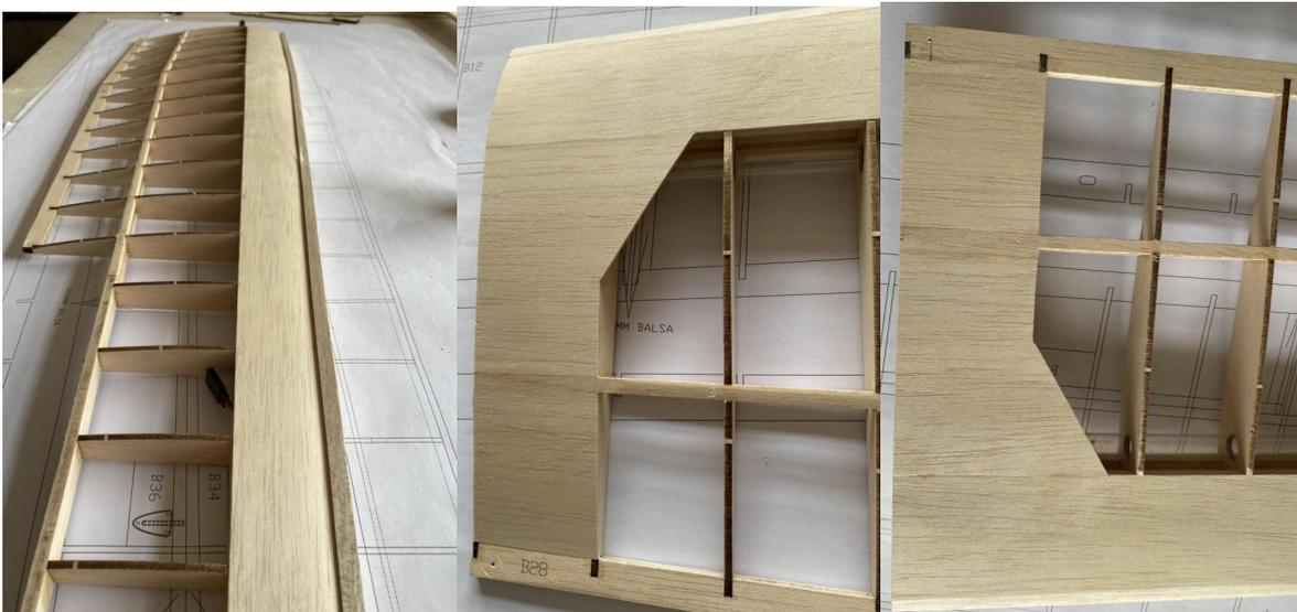
11) Polish front and rear edges of wings while using paper tape as a precaution against over-polishing.
