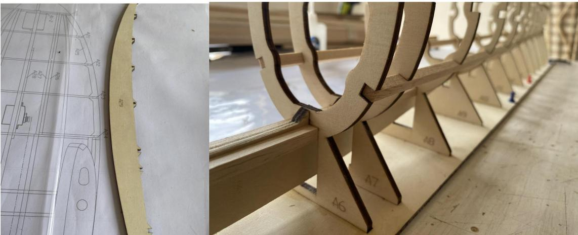
6) Glue balsa sheets to both upper and lower sections, as well as both sides of the fuselage (**B1 is used for temporary positioning of partition bulkheads A6, A7, and A8; refrain from gluing at this stage. B1 will be glued at step 17**).
