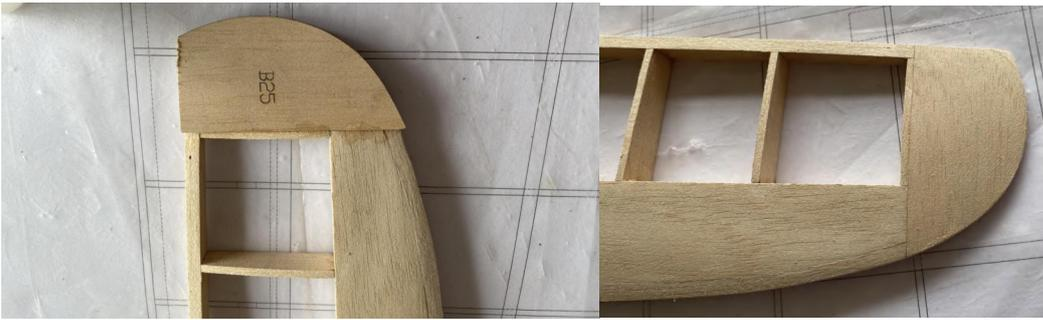
**13) Install aileron servo mount, glue 2MM balsa on the top, then strengthen by gluing pine block.**
