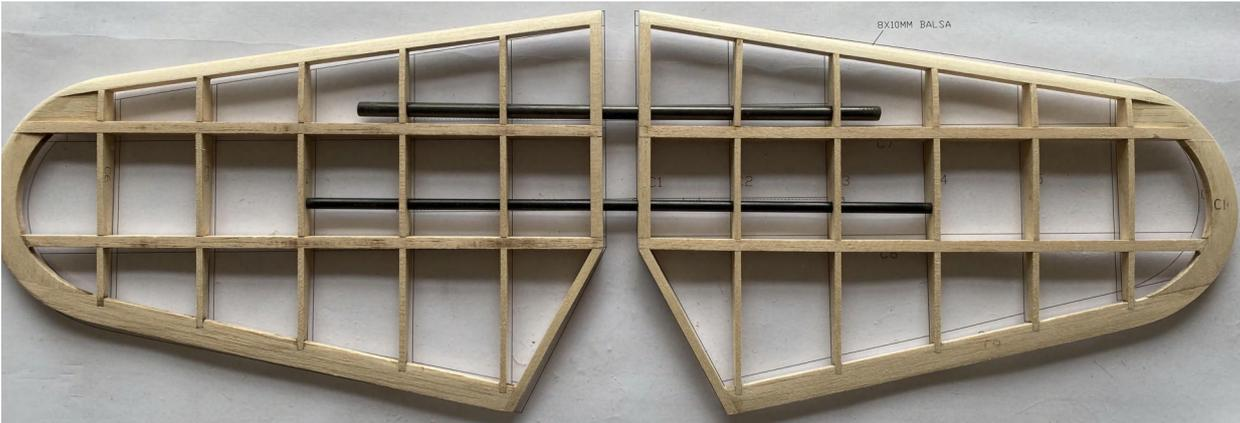
**4) Assemble main beams according to their numbers, then glue wing ribs accordingly.**
