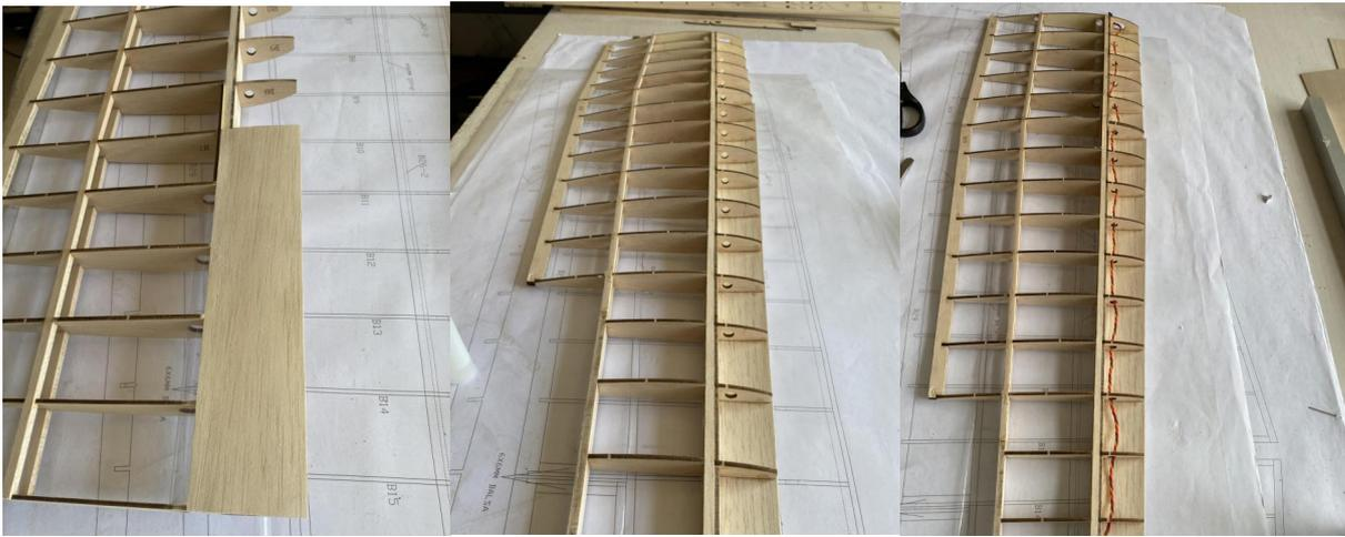
10) Glue 8MM balsa on leading edge of wings and 2MM balsa cover in middle section of wings.
