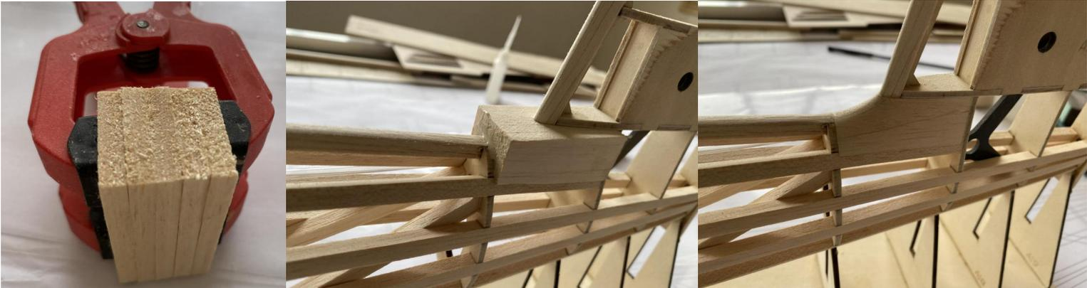
13) Install elevator pulling connecting rod and clevis, **seal fuselage sides** with 3MM balsa sheets.
