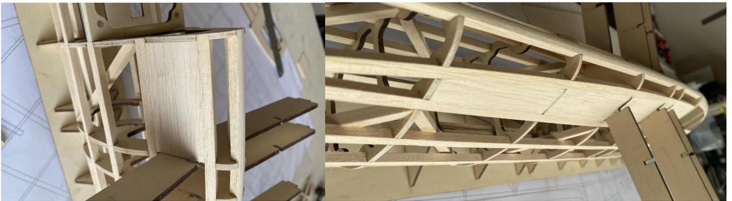
17) Glue B1 to the fuselage, ensuring that the balsa sheets are drilled to accommodate the servo extension wires.
