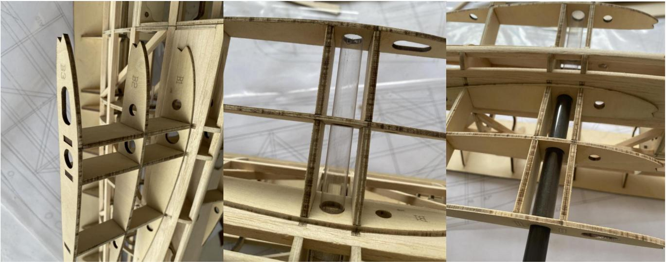
19) Glue 8X8MM balsa strips to the leading edge and then glue 2MM balsa cover.
