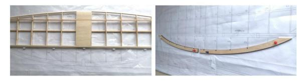
(34) Glue 10X8mm balsa strips and wing ribs.
