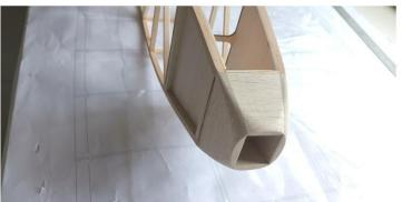
(17) Install magnets on the battery cover and mount, and stick the battery mount to the bulkhead of the fuselage.
