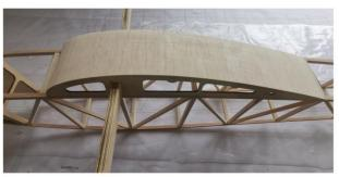
(14) Glue the horizontal tail wing supportor and glue the stiffener, then glue servo mount numbered A7 to the fuselage.
