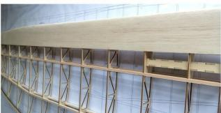
(27) The balsa strips on the trailing end of the wings need to be remove 2mm,in order to balance the balsa cover for the upper and lower of the trailing end of the wings.
