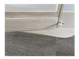
(39) Install self–tapping screws and fix with rubber bands.
