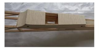
(16) Combin and glue the nose and glue it to the fuselage.
