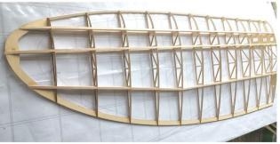
(25) Combine the wing joint boxes and glue it to the wing ribs.
