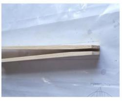
(6) Make the fuselage fixture with the laser–cut plywood and fix it in accordance with the position on the plan.
