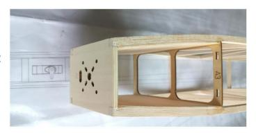
(10) Glue A4 into the fuselage, and combine and glue the wing joint parts, then glue it on A4 according to the position marked on A4.
