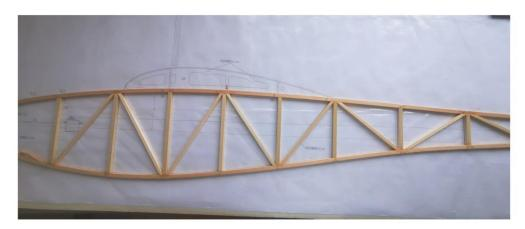
(3) Strengthen the nose part with 3mm balsa strip. Pay attention to the symmetrical adhesion on both sides of the fuselage.
