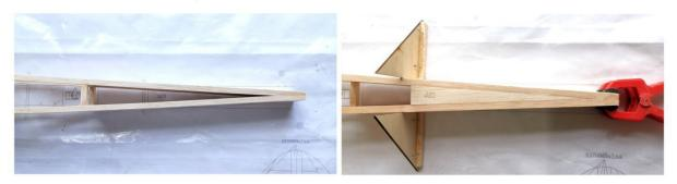
(9) Glue the motor mount numbered A1 inside.
