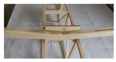
(11) Glue bulkhead numbered A6 to the fuselage, and glue the two
