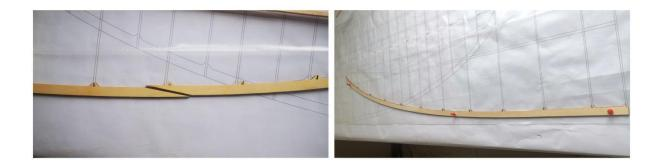
(22) Glue the wing ribs and balsa strips accoding to the plan.
