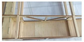
(28) Glue the balsa cover for the trailing end of the wings, making sure the B1 ribs are flat (otherwise the wings will connect to cause large gaps).
