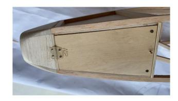
(19) Glue wood strips inside the battery compartment, and fix the battery fixing plate with screws.
