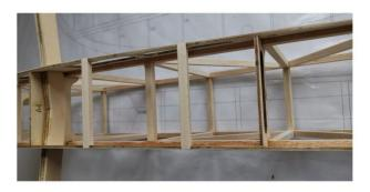
(13) 2mm balsa sheet covered on the wing supportor.
