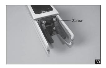
2. Locate the long piece of wire used for the throttle pushrod. One end of the wire has been pre-bend in to a "Z" bend at the factory. This "Z" bend should be inserted into the throttle arm of the engine when the engine is fitted onto the engine mount. Fit the engine to the engine mount using the screws provided.
