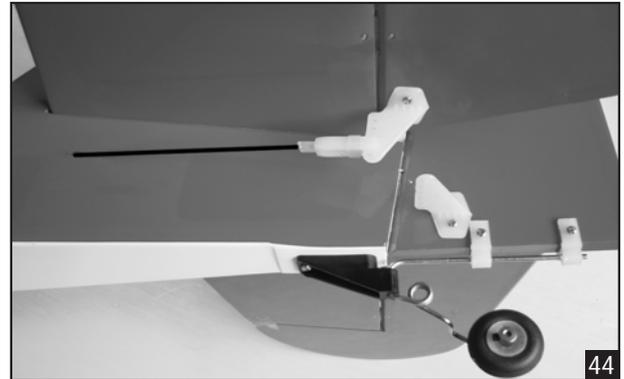
7. Attach clevis to the third hole in the control horn. Install a silicone tube on the clevis.
