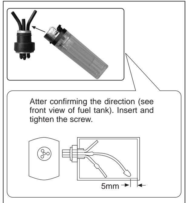
5. Test fit the stopper assembly into the tank. It may be necessary to remove some of the flashing around the tank opening using a modeling knife. If flashing is present, make sure none of it falls into the tank.
