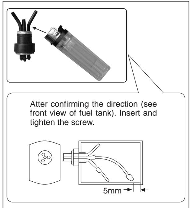
After confirming the direction (see front view of fuel tank). Insert and tighten the screw.
