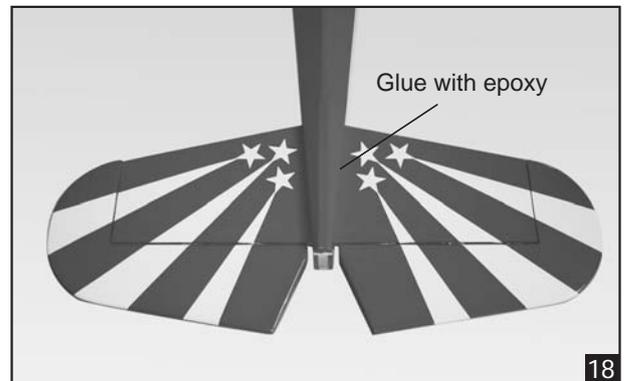
7. After the epoxy has fully cured, remove the masking tape or T-pins used to hold the stabilizer in place and carefully inspect the glue joints. Use more epoxy to fill in any gaps that were not filled previously and clean up the excess using a paper towel and rubbing alcohol.
