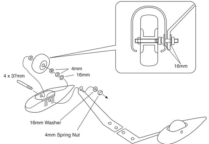
**!** After installing the wheel pant, apply a small drop of thin C/A to the bottom nut.
