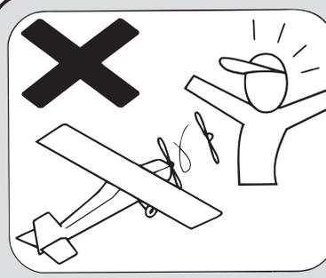
**ALWAYS** adjust the engine from behind the propeller, and do not allow any part of your body to be in line with the propeller.
