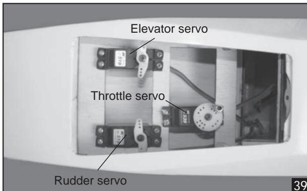
**INSTALLING THE ELEVATOR PUSHROD**
