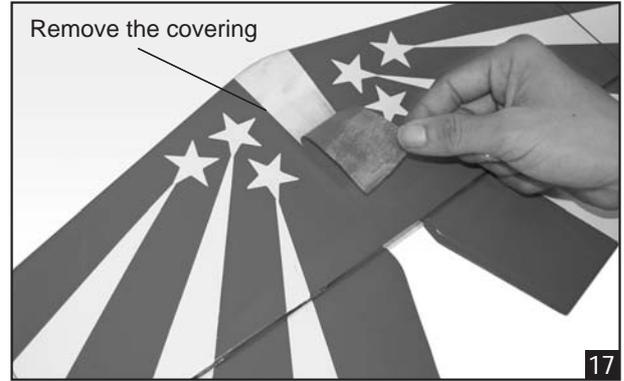
6. When you are sure that everything is aligned correctly, mix up a generous amount of 30 minute epoxy. Apply a thin layer to the top and bottom of the stabilizer mounting area and to the stabilizer mounting platform sides in the fuselage. Slide the stabilizer in place and re-align. Double check all of your measurements one more time before the epoxy cures. Remove any excess epoxy using a paper towel and rubbing alcohol and hold the stabilizer in place with T-pins or masking tape.
