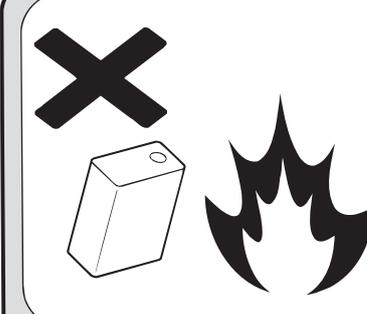
**DO NOT** dispose of empty fuel containers on a fire, this can lead to an explosion.
