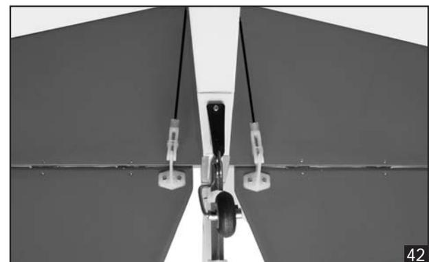
8. Locate one nylon servo arm, and using wire cutters, remove all but one of the arms. Using a 2mm drill bit, enlarge the third hole out from the center to accommodate the elevator pushrod wire.
