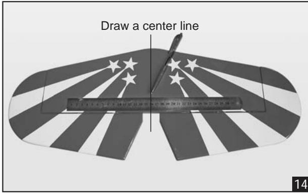
3. Check the fit of the horizontal stabilizer in its slot. Make sure the horizontal stabilizer is square and centered to the fuselage by taking measurements, but don't glue anything yet.
