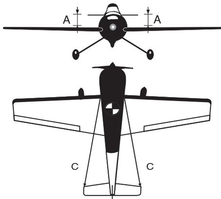
4. With the horizontal stabilizer correctly aligned, mark the shape of the fuselage on the top and bottom of the tail plane using a water soluble / non-permanent felt-tip pen.
