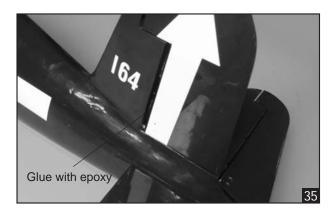
8. Glue the C.A hinge rudder by C.A glue.
