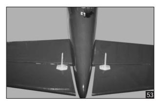
7. Attach clevis to the third hole in the control horn. Install a silicone tube on the clevis.
