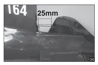
7. Insert and glue the tail gear to the rudder using epoxy glue.
