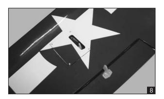
3. Repeat step # 1 - # 2 to install the control horn on the opposite aileron.
