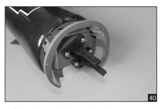
2. Place the engine into the engine mount and align it properly with the front of the cowling. The distance from the firewall to the front of the engine thrust washer should 110mm.
