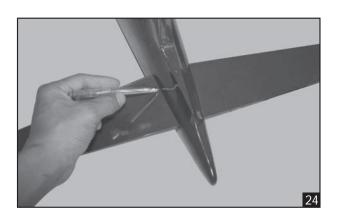
5. Remove the stabilizer. Using the lines you just drew as a guide, carefully remove the covering from between them using a modeling knife.
