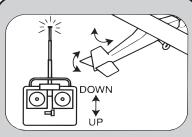
Operate the control sticks on the transmitter and check that the control surfaces move freely and in the CORRECT directions.
