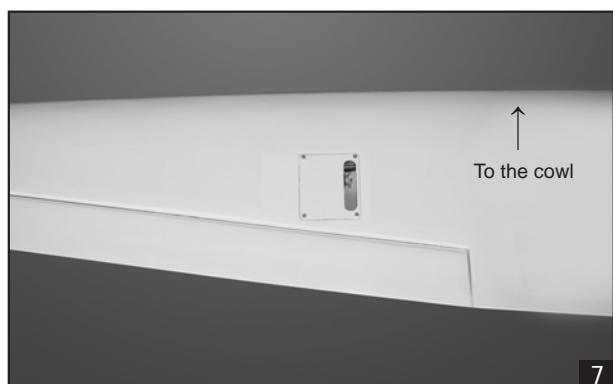
7. Using masking tape, tape the servo leads on to the top of the wing.
