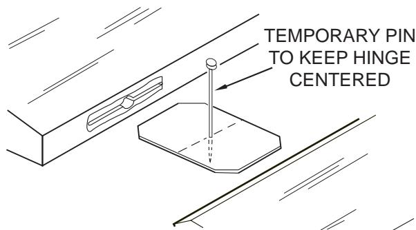
5. Apply six drops of thin CA to the top and bottom of each hinge. Do not use CA accelerator. After the CA has fully hardened, test the hinges by pulling on the aileron.
