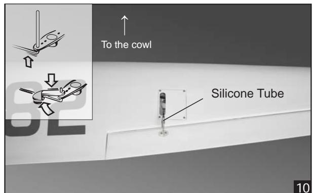
9. Repeat step # 4 - # 8 to install the second aileron linkage. After both linkages are completed, connect both of the aileron servo leads using a Y-harness you have purchased separately.
