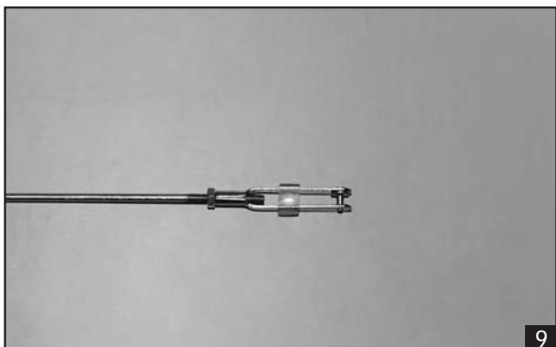
2. Attach the clevis to the outer hole in the control horn. Install a silicone tube on the clevis.
