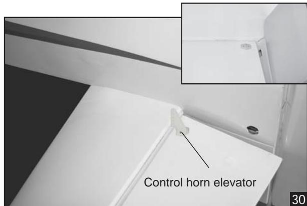
**INSTALLING THE ELEVATOR PUSHROD**
