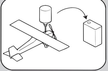
Empty the fuel tank after flying, fuel left in the tank can cause corrosion and lead to engine problems.
