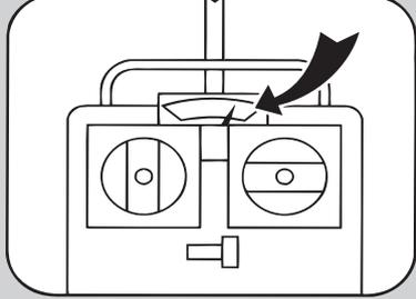
Check that the transmitter batteries have adequate power.
