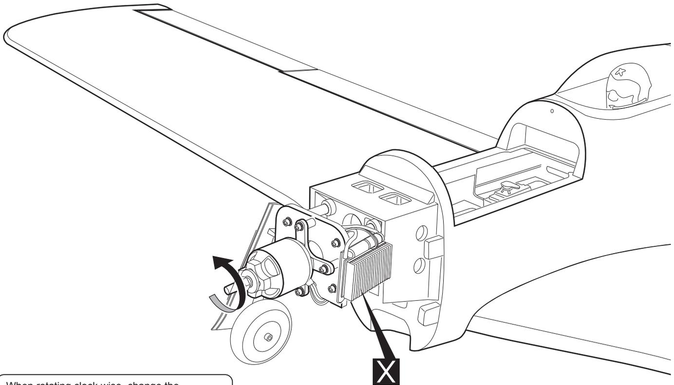
When rotating clock wise, change the connection of 2 wires.
