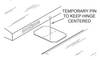
2. Apply six drops of thin CA to the top and bottom of each hinge. Do not use CA accelerator. After the CA has fully hardened, test the hinges by pulling on the aileron.
