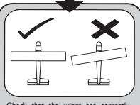
Check that the wings are correctly fitted to the fuselage.
